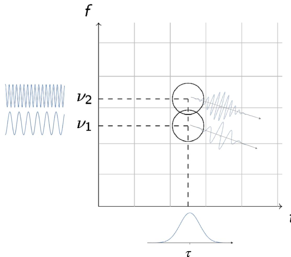
**Gabor Decomposition.** The atoms used are now localized both in time and in frequency, but are spread on the time-frequency plane.
