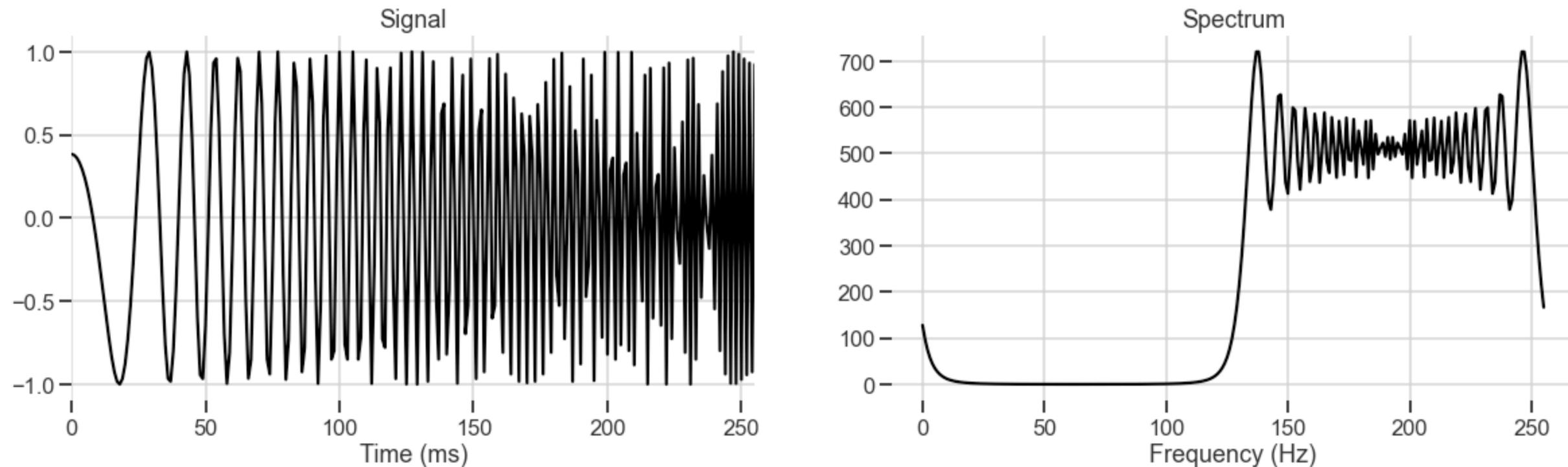
**Limitations of spectral analysis.** Here we perform a spectral analysis of a *chirp* (left), which is a signal whose frequency is linearly modulated over time. Think to a *slide-whistle* or  $\cos(\omega t \times t)$ . The resulting spectrum (right) is hard to analyze and does not really capture the underlying notion of *instantaneous frequency*.
