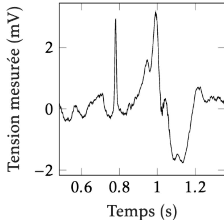
**Left.** An artefact at  $t \approx 0,8s$  followed by two simultaneous HFO (ripple and fast-ripple) at  $t \approx 1s$ .
