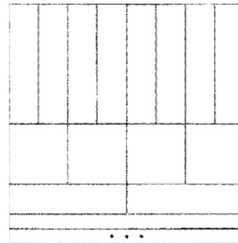
**Wavelet Decomposition.** Atoms are affine dilation of a common oscillatory element (+ time shifted).
