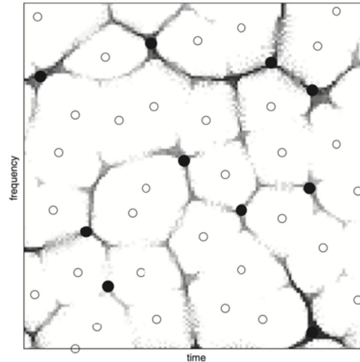
**Reassigned Spectrogram of White Noise.** Voronoi-diagram like structure are exhibited when following the reassignment field. The zeros are represented as the white circles.
