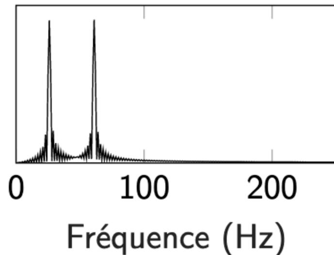
**Limitations of spectral analysis.** Here two signals are spectrally analyzed. The first one is a succession of 0,25s of 25Hz oscillations and 0,25s of 60Hz oscillations. The second one is time reversed. The Fourier analysis, when analyzing this signal on all its duration is unable to distinguish the two (if we restrict ourselves to the amplitude of its coefficients).
