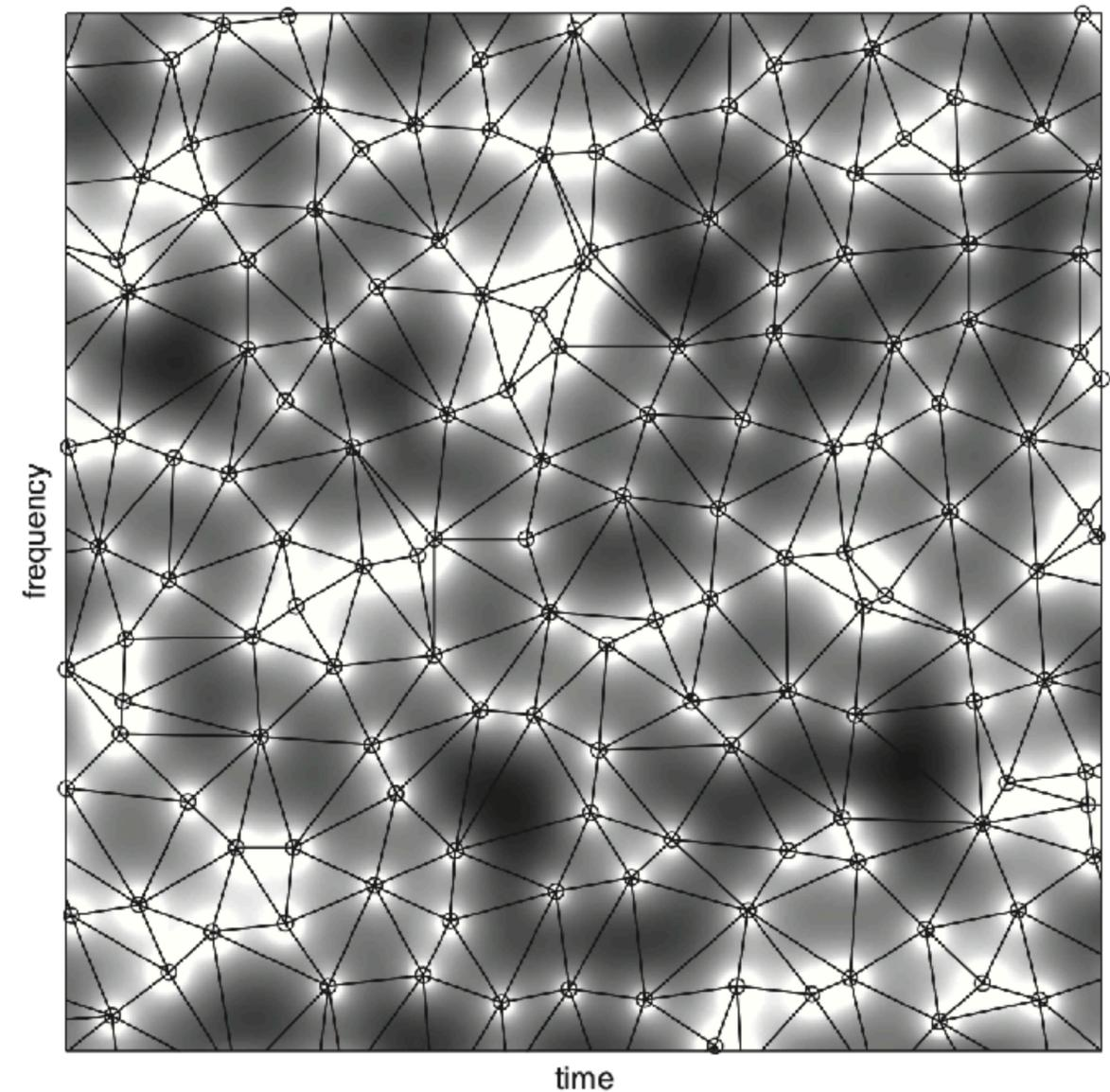
**Delaunay Triangulation.** The Delaunay triangulation is a dual structure of the Voronoi tessellation. The Delaunay triangulation of packed logons is expected to be composed of quasi-equilateral triangles.
