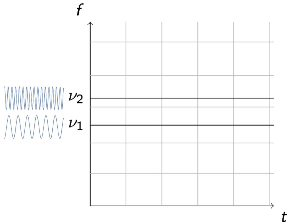
**Fourier Transform.** The atoms used are perfectly localized in frequency, but not at all in time.
