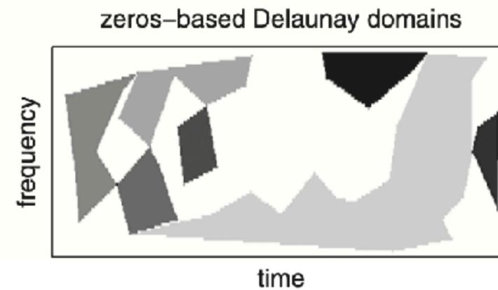
**Zero-based filtering of the GW150914 event (gravitational waves)**
