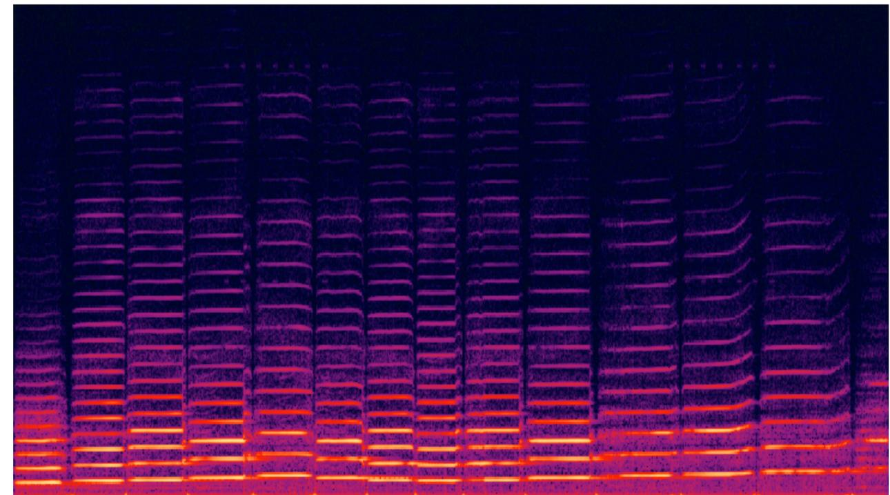
**A spectrogram of a violin waveform.** Created by [User:Omegatron](#) for Wikimedia.
